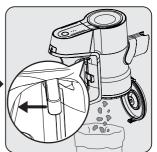
Pull the emptying dust container trigger to the last point. Dust container lid will be opened. Empty all the dust it contains.
