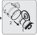
To take out the plastic filter, first rotate the plastic filter counter clockwise (1), then pull out the filter (2).
