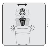
Remove the dust on the pre-filter and the plastic filter by tapping it on a hard surface such as a waste bin or by using a brush.
