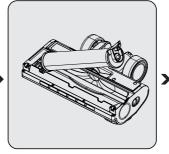
Remove the dust on it by tapping it lightly to a hard surface or remove the dust with a brush. If any hair, etc. is tangled, remove it by cutting it off.
